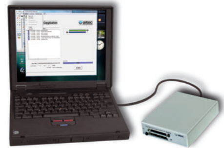
FlashCard CopyStation Mobile connected to a Notebook or a PC via USB
